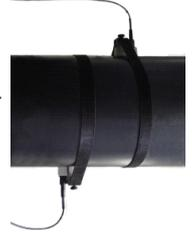
WPG, XPG, YPG and YPGD transducers operate in transit time mode and are for clean fluid applications. The YPG transducers are especially good with lined pipes\* and applications above 100mm.
